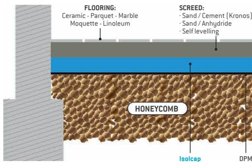
**BETWEEN FLOORS: INTERMEDIATE LIGHTWEIGHT AND THERMAL INSULATING LEVELLING LAYER**
